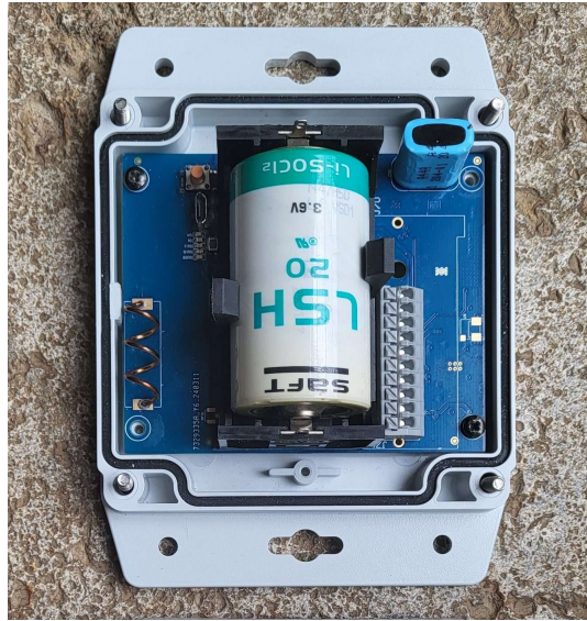
A single Type-D lithium battery powers the SV2 actuator – observe the polarity marked on the holder
